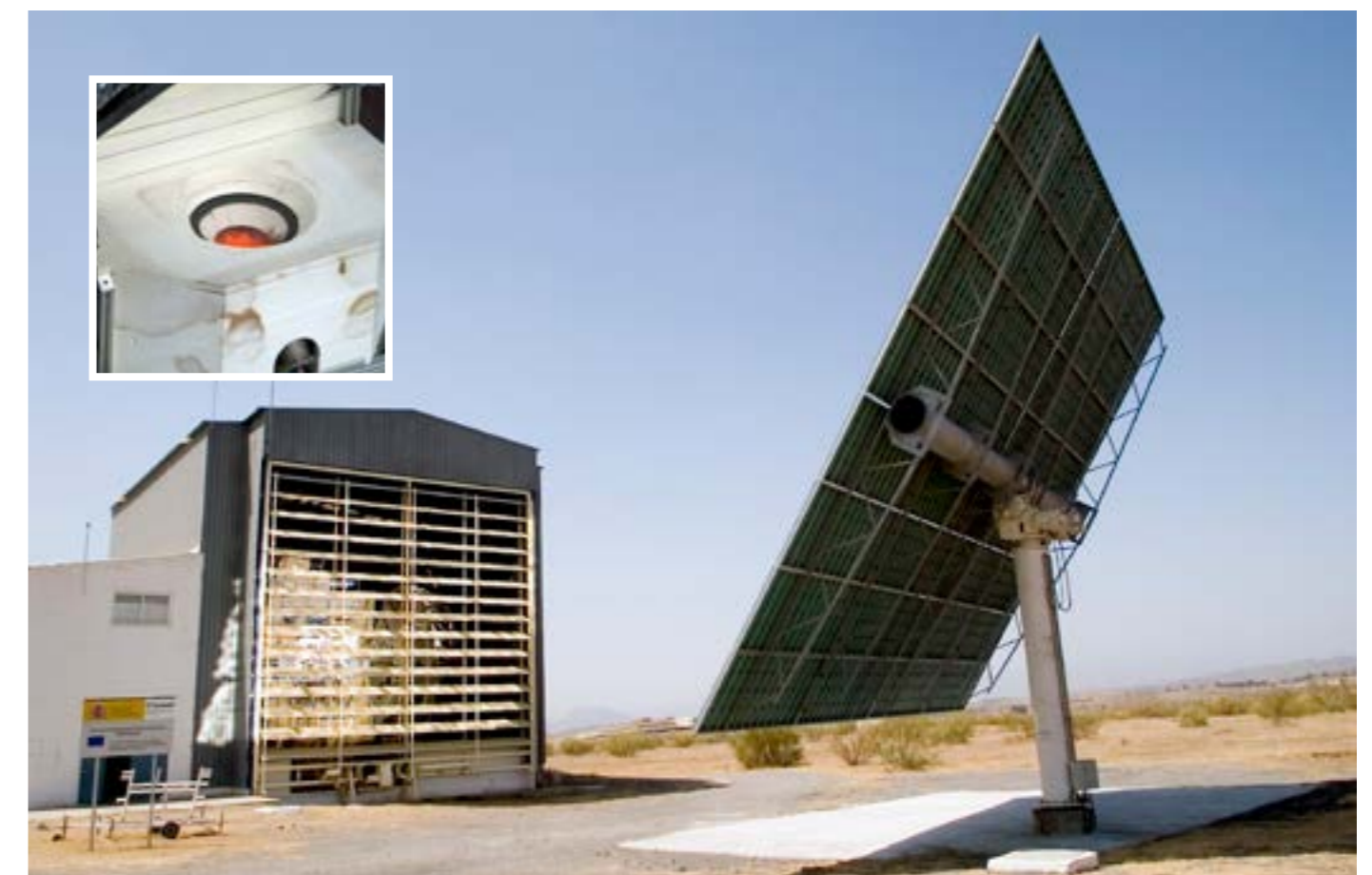
Upper left box: red hot fluidized bed after solar test of lunar regolith reduction at the Solar Furnace of the Plataforma Solar de Almería
